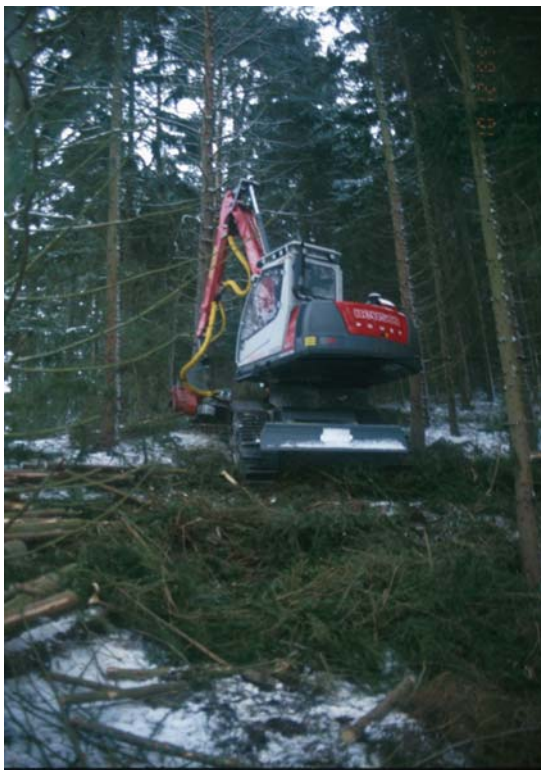
Abb. 4: Raupenharvester Neuson 11002 HV (Photo: LWF)
