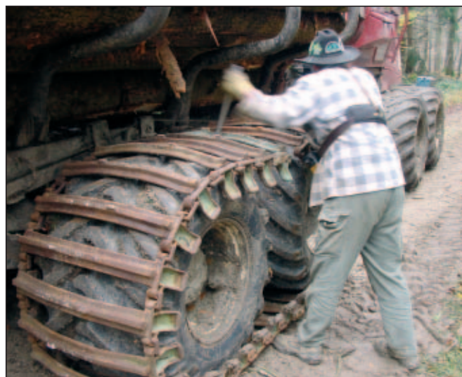
Abb. 2: Montage des Bogiebandes Eco-Track (Foto: J. Kremer)
